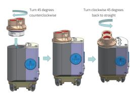
Turn the lamp head 45 degrees counterclockwise and insert it into the main body, then turn it 45 degrees clockwise and return it to the straight position before assembly is complete. Remember to distinguish the front and bottom surfaces when assembling the lamp head.
